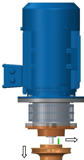
3. Remove impeller (2) and key (19)
